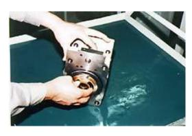
3.3.13. Remove the needle bearing (124) and spline coupling (114) from the valve block (312).
